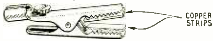
Fig. 5. Thermal shunt made from a crocodile clip as explained in the text.
