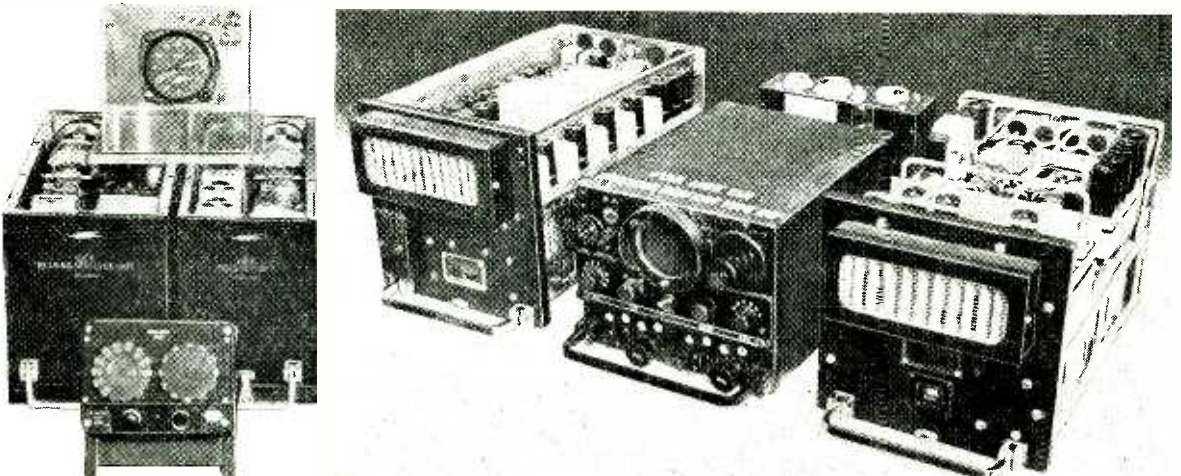
Standard Telephones VOR aircraft receiver and associated units and (right) Cossor Radar lightweight Mark III Gee aircraft receiver.
